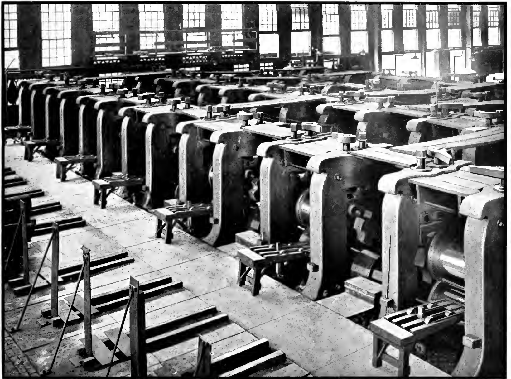
Mesta Cold Mills for Tin Plate Installed at The McKeesport Tin Plate Company
